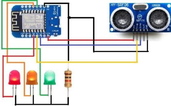
Figure 5 - Connectivity within each parking sensor
