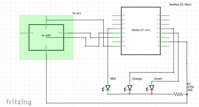
Figure 6 - Schematic Diagram of each parking sensor
