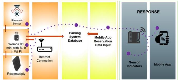
**Figure 1. The Input-Process-Output (IPO) of the system, showing the flow of information**
