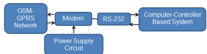
Figure 1. Block Diagram of GSM Module
